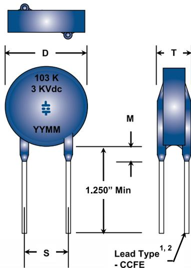
**CalRamic Technologies LLC** manufactures a series of highly reliable, single layer, conformally coated, negative temperature compensating, leaded ceramic disc capacitors that deliver both very stable and predictable performance characteristics typically associated with low loss dielectrics.
